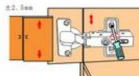
MOUNTING PLATE IS ENABLE FINE TURNING TO ADJUST THE DOOR UP AND DOWN
